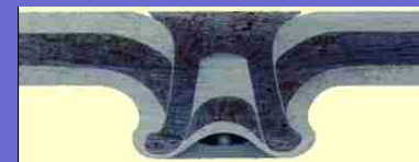
aluminium - 1.2mm, stal - 1.8mm, aluminium - 1.2mm
