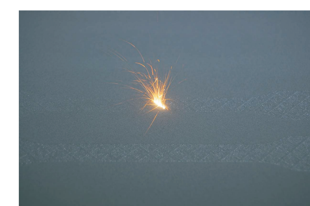
Rys. 18. Proces SLS - spiekanie proszku Ti6Al4V w komorze roboczej Fig. 18. SLS process - sintering of Ti6Al4V powder in the working chamber
