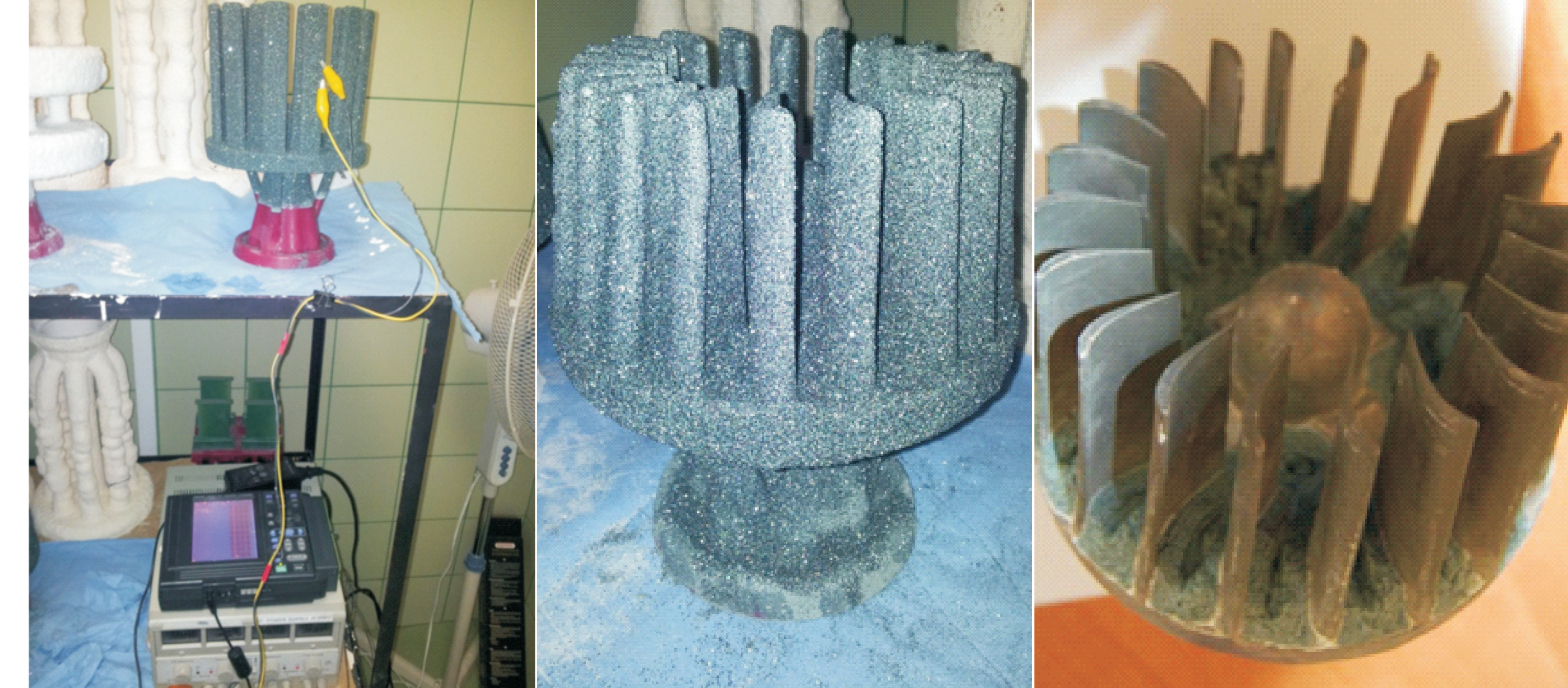
Stanowisko do badań kinetyki suszenia formy Installation for investigation of mold drying kinetics
