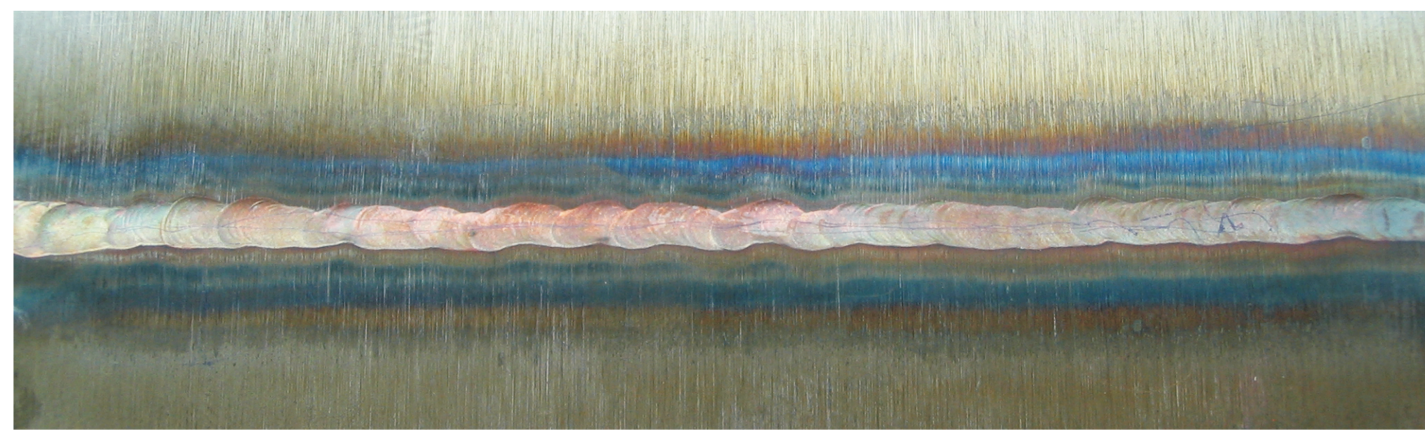
Rys. 2. Spoina wykonana metodą TIG bez dodatku spoiwa. Fig. 2. Fusion weld made by TIG method without added metal.
