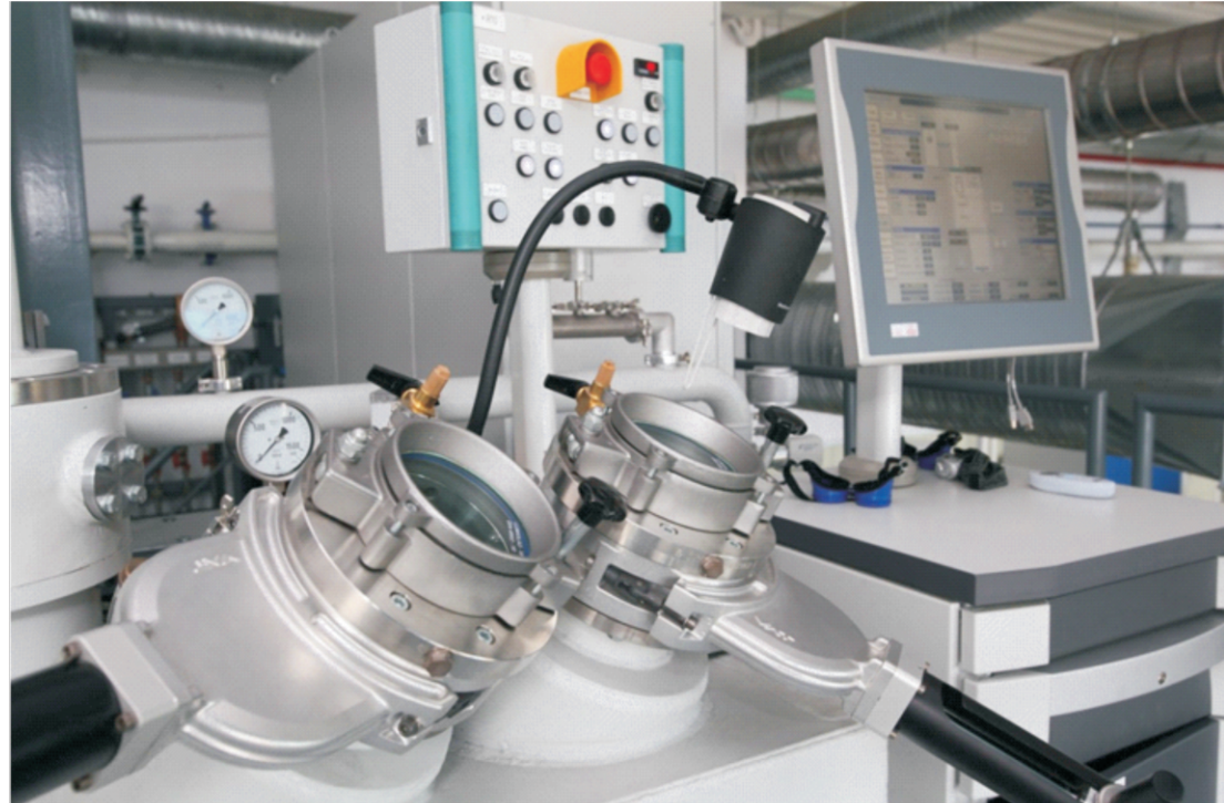
Rys.8. Piec do wytwarzania monokryształu VIM-IC 2E-DS/SC firmy ALD Fig. 8. VIM-IC 2E-DS/SC investment casting furnace by ALD Vacuum Technologies for single crystal casting
