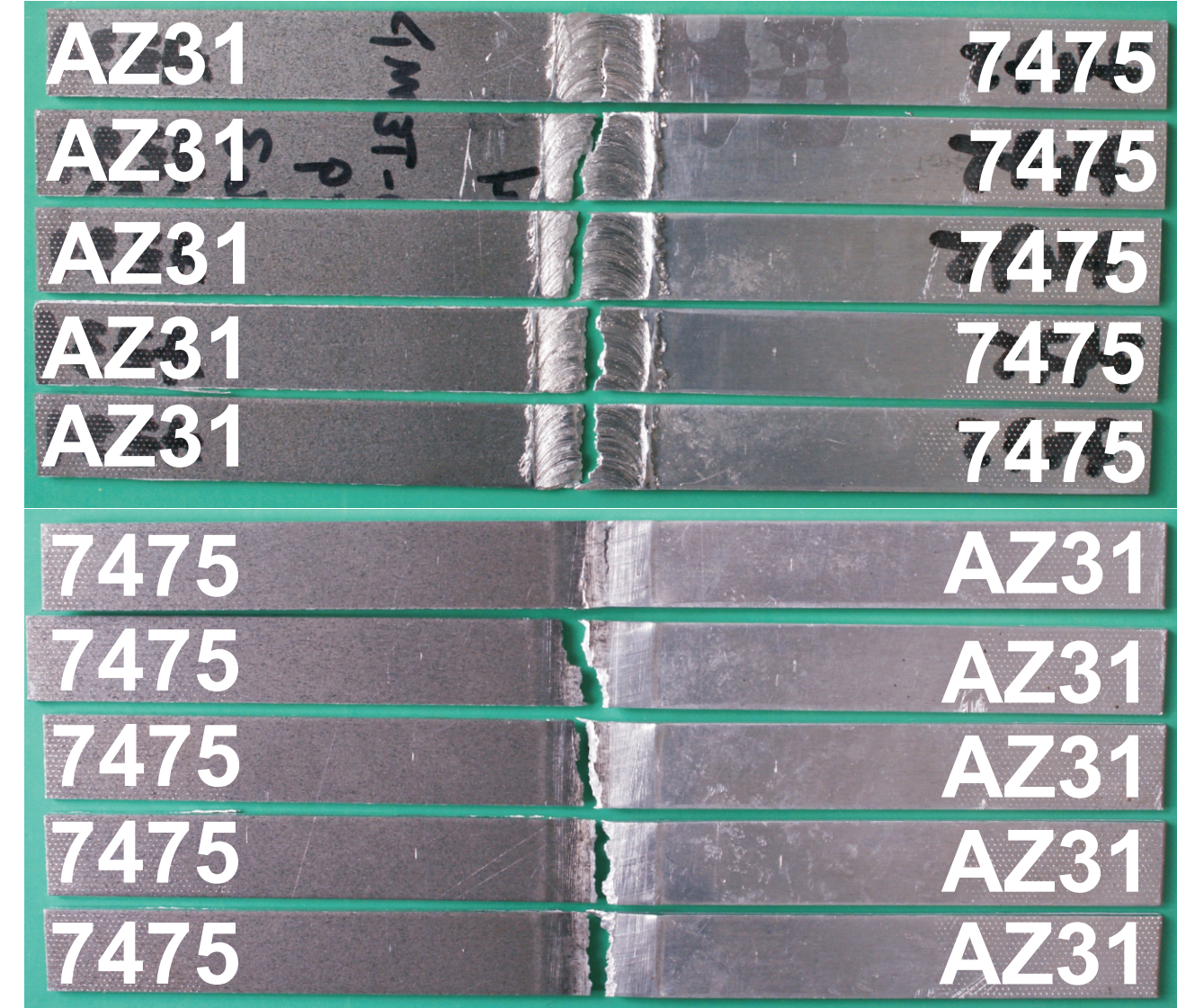
Rys. 13. Charakterystyki mechaniczne złączy FSW stopów magnezu AZ31 i aluminium 7475 Fig. 13. Mechanical characteristics of the FSW joints of magnesium alloy AZ31 and aluminum alloy 7475
