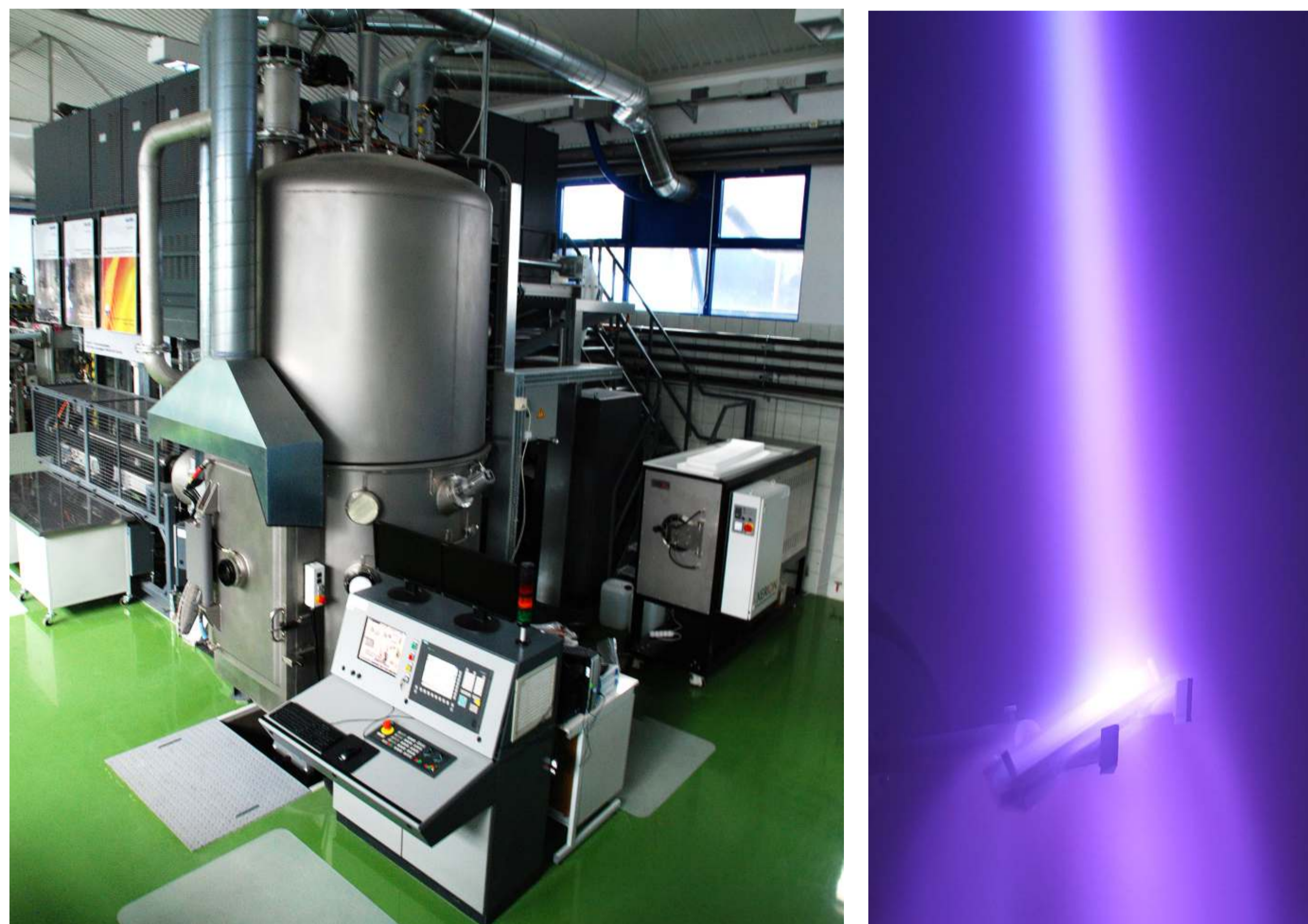
System do osadzania powłok metodą PS-PVD The equipment for deposition of ceramic coatings by PS-PVD method
