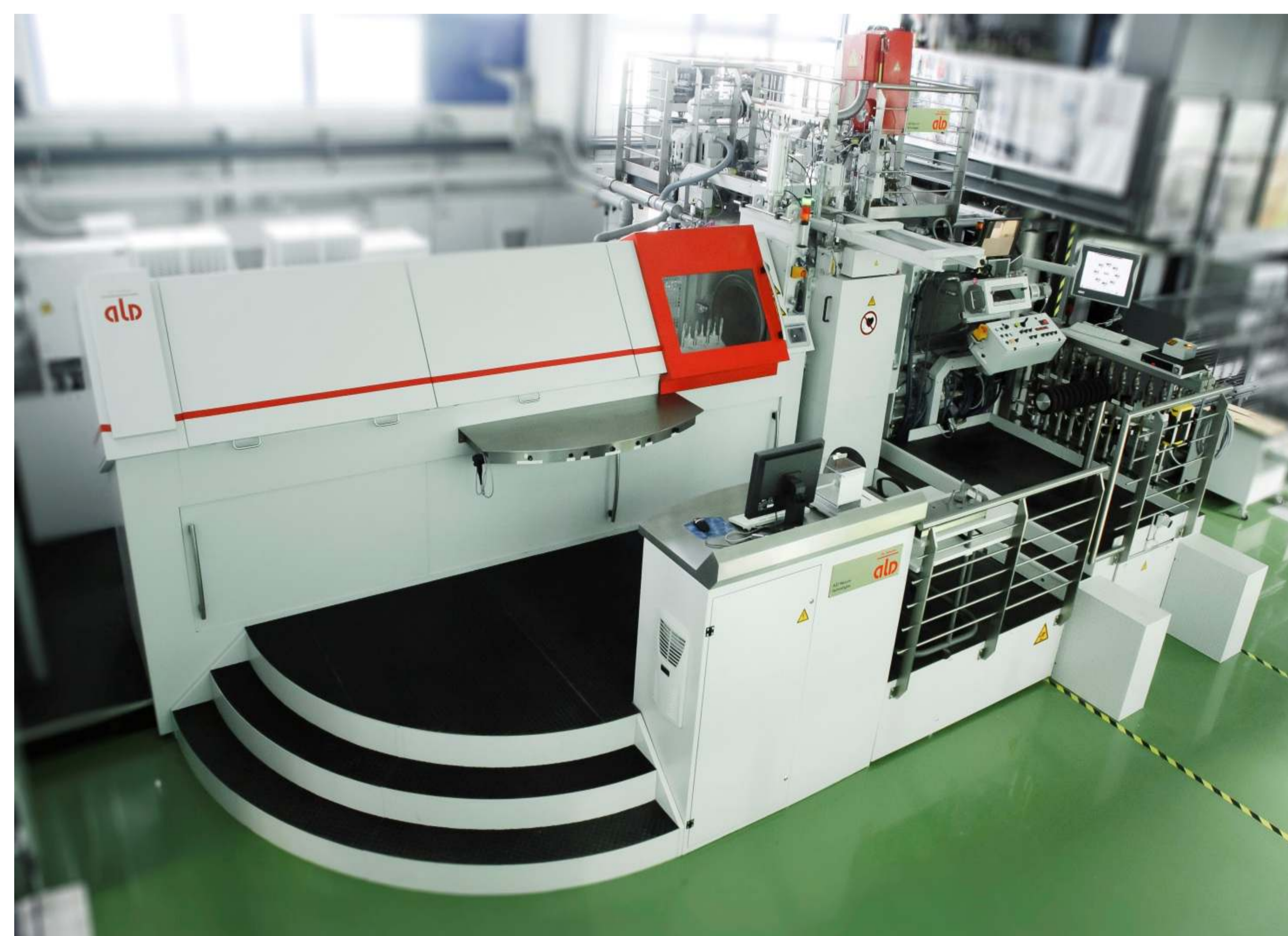
System do osadzania powłok metodą EB-PVD The equipment for deposition of ceramic coatings by EB-PVD method
