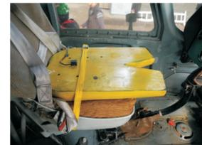
Rys. 16. 77,5 kg RCLI type indenter placed on the pilot seat
