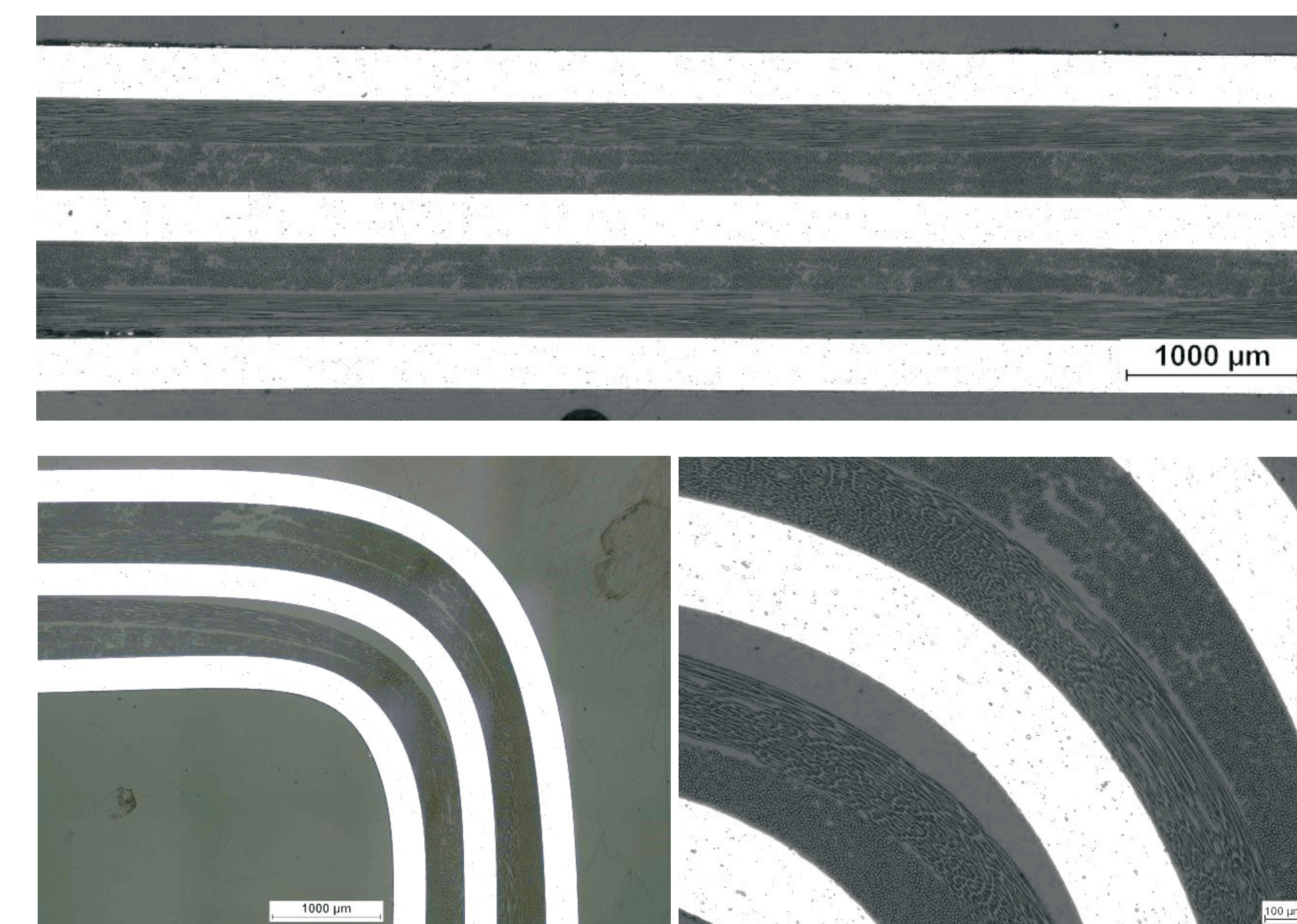
Rys. 6. Mikrostruktura profili FML Fig. 6. microstructure of FML profiles
